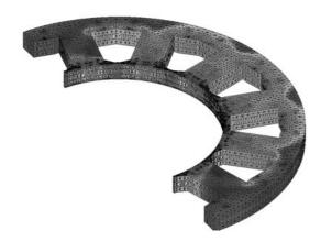
Fig. 3: 3D electromagnetic analysis (1/2 model of the distribution for magnetic flux density of the stator core)
