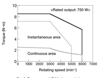
Fig. 9: Torque speed (T-N) characteristics (Flange dimensions: 80 mm) (Dotted lines indicate specifications from previous SANYO DENKI models)
